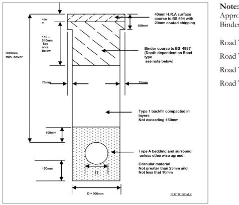
Appropriate depth of Bindercourse Material Road Type 1: 310mm Road Type 2: 245 mm Road Type 3: 150 mm Road Type 4: 110 mm
