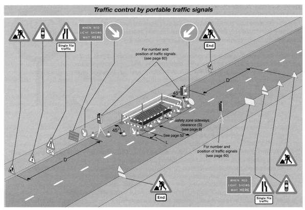
For numbers and size of cones, length of lead in taper (T) and dimensions 'D', 'L' and 'S', see table below. Information boards should also be displayed (although omitted here for clarity)
