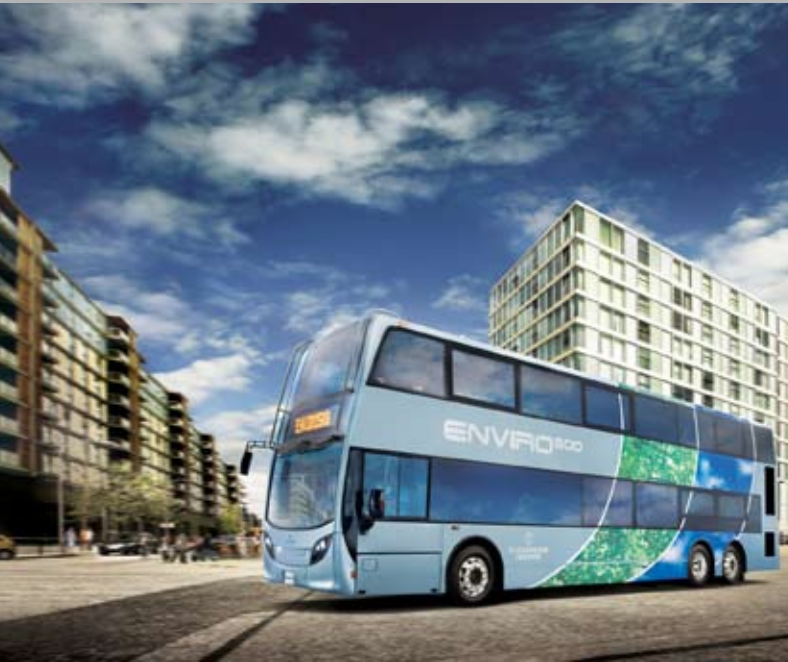
ADL's new three-axle double deck for export markets. Known as the Enviro500 it can carry 100 passengers.
