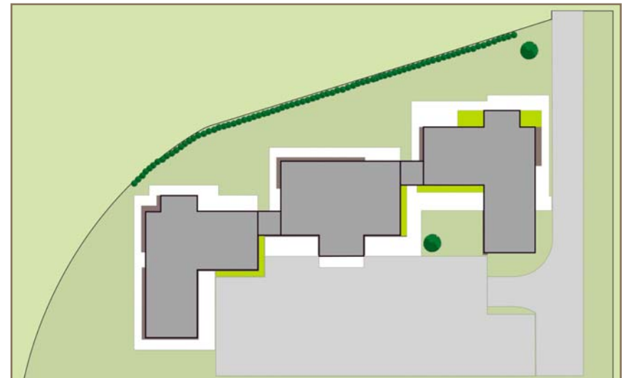
Regular Urban Arrangement is inappropriate in a Rural Setting
