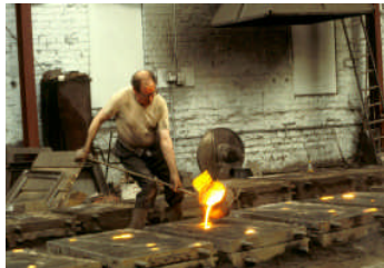
Pouring molten iron into moulds at New Grange Foundry (Ballantines), Bo'ness, 7th August 1979
