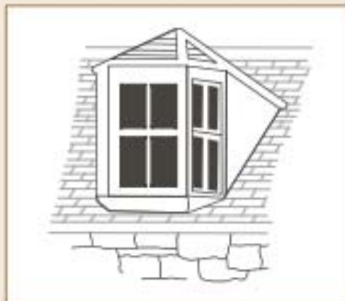
Figure 19d : DORMER WINDOW TYPES Angled Bay/Hipped Roof
