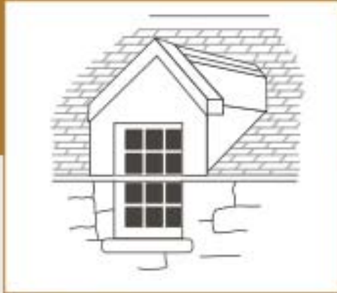
Figure 19a : DORMER WINDOW TYPES Wall Head/ 1 st Storey
