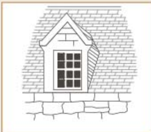
Figure 19b : DORMER WINDOW TYPES Wall Head
