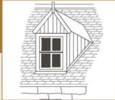
Figure 19c : DORMER WINDOW TYPES Straight Gable
